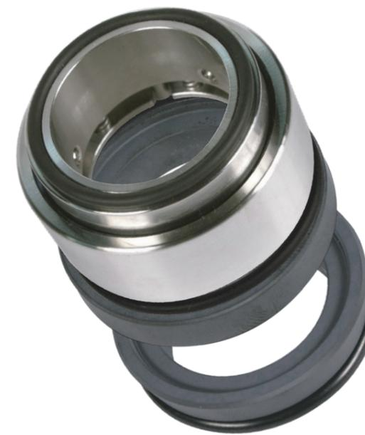
For applications where the sealing faces of the mechanical seal are poorly lubricated, Packo Pumps developed the Novapad seal. Its seal faces consist of specially treated silicon carbide to adjudge self lubricating properties whilst maintaining the same hardness and durability of silicon carbide.
