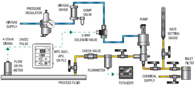
(1) Note: the controller would not be used with the solenoid valve.
