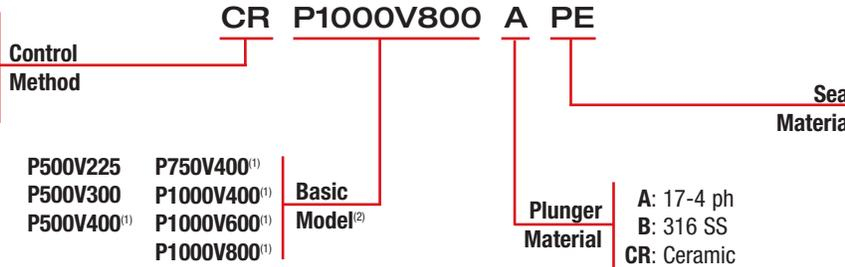
**NOTE:** <sup>(1)</sup> The 400, 600 and 800 motor cylinders are only available with the CR (controller-relay) or SR (solenoid-relay) control methods.
