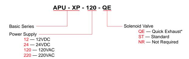
\*Quick Exhaust (QE) option is used when maximum number of strokes are required on larger sized pumps.
