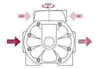
Orientable air inlet, increased installation flexibility.
